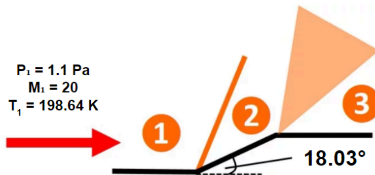
Figure 9: Oblique shock followed by expansion fan
