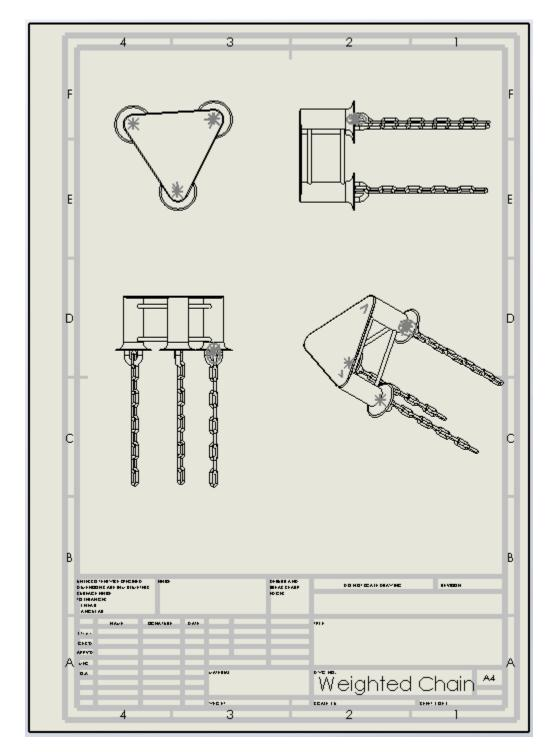
SolidWorks drawing of Principle Power Base with weighted chains
