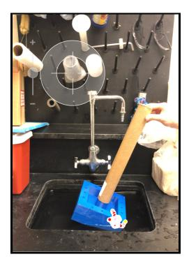
A number of modifications were made to the bases in order to test different concepts for achieving better stability. Chains were attached to the Principle Power base, as well as styrofoam to the legs. A number of tests were run in different configurations. Weights were added to the corners or hung from the bottom of the Naturally Pressurized Base.
