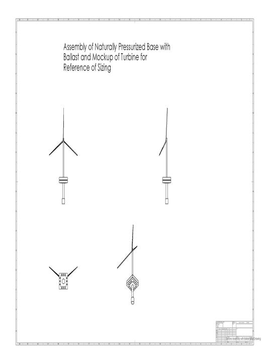
SolidWorks drawing of Naturally Pressurized Base with a mockup of turbine blades for reference
