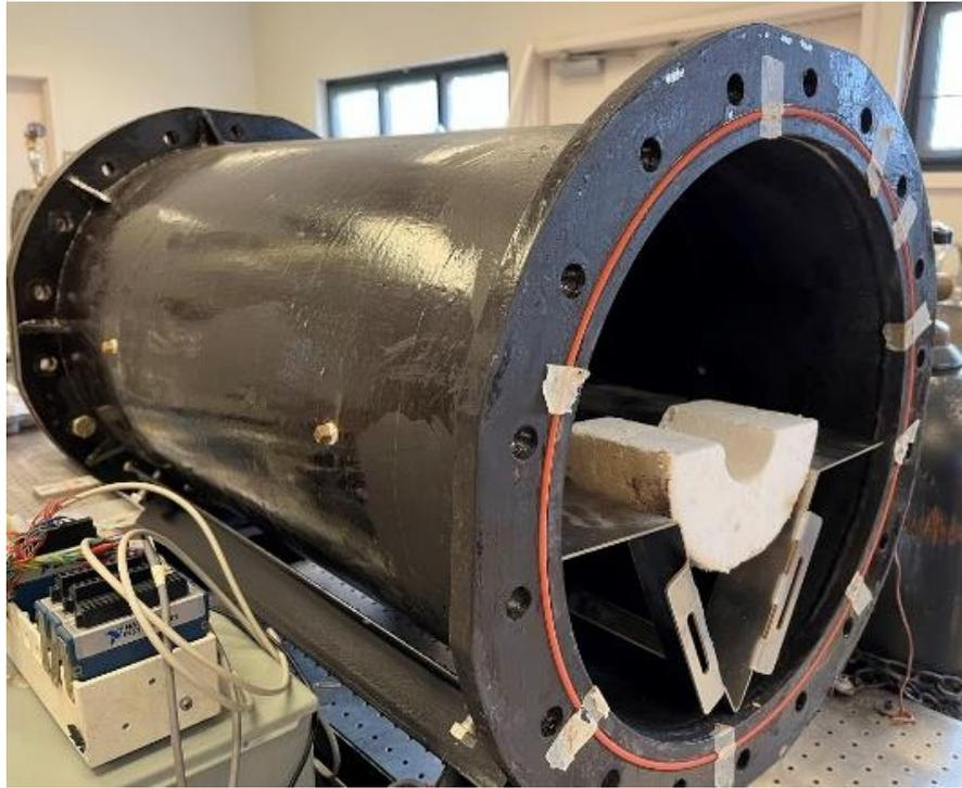
Figure 3.4: New high-pressure enclosure with 16” ID and 30” length, with provision for sliding in and out the modular heaters mounted on a V-shape trough.
