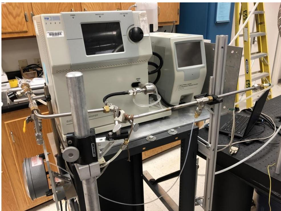
Figure 3.3: Image of the portable SMPS setup with 250 $\mu$ m probe orifice mounted on an equipment rack.
