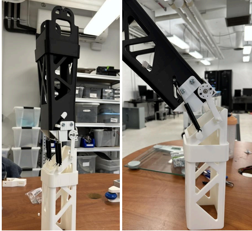
Fig. 33: Image of a passive and half-bent leg with the damping system
