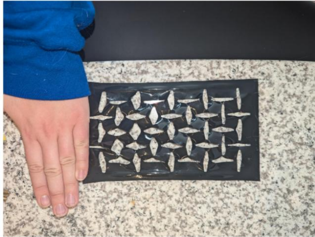
Figure 15. Large scale prototype stretching of rounded kirigami substrate to 10% deflection.
