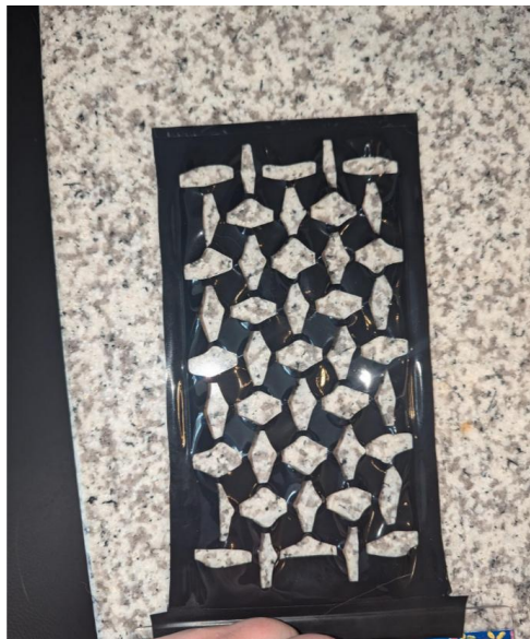
Figure 16. Large scale prototype stretching of rectangular kirigami substrate to 10% deflection.
