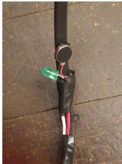
Figures #12 and #13: Sensor and vibration motor attached to headphones
