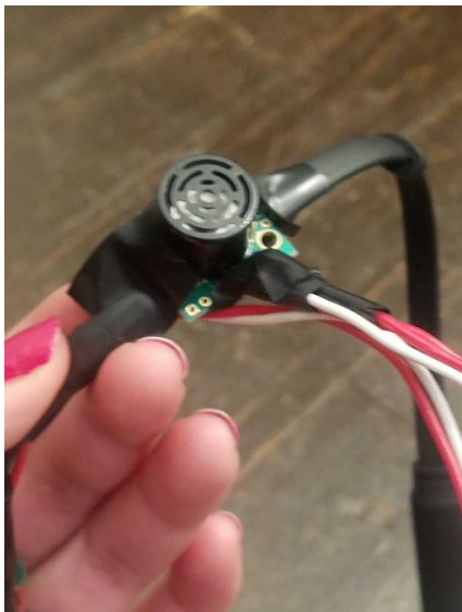
Figures #12 and #13: Sensor and vibration motor attached to headphones
