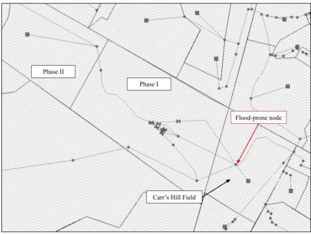
**Figure 16.** SWMM model produced by Biohabitats, Inc. showing downstream pipes, junctions, and other stormwater structures. The Phase I infrastructure is post-redevelopment and Phase II is pre-redevelopment. The flooding node is indicated by the red arrow.
