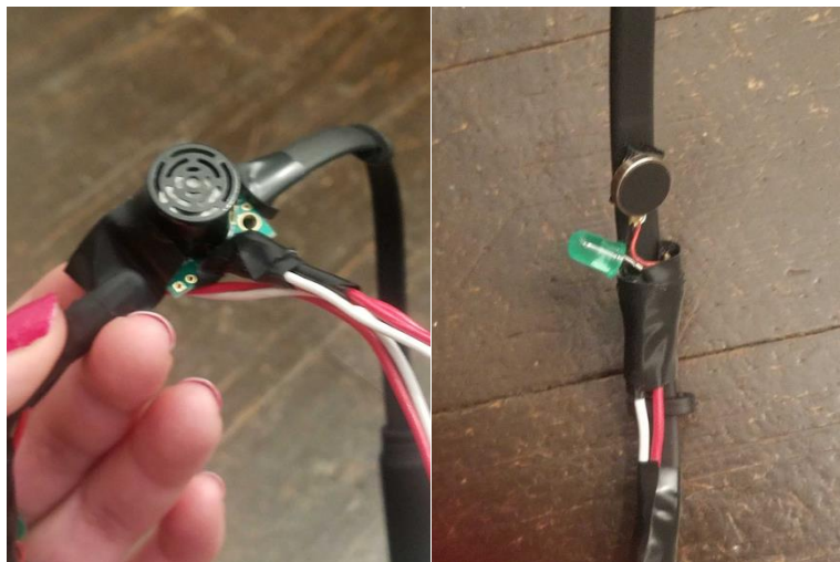
Figures #12 and #13: Sensor and vibration motor attached to headphones
