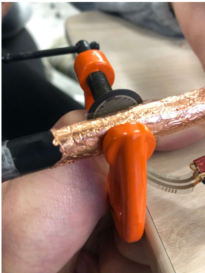
Fig. 4. Experimental setup for measuring a constant force applied to both the FSR on a Cook Aortic Endograft and a FlexiForce sensor. constant force was simultaneously applied to both sensors using a C-clamp and the voltage outputs for both sensors were recorded.
