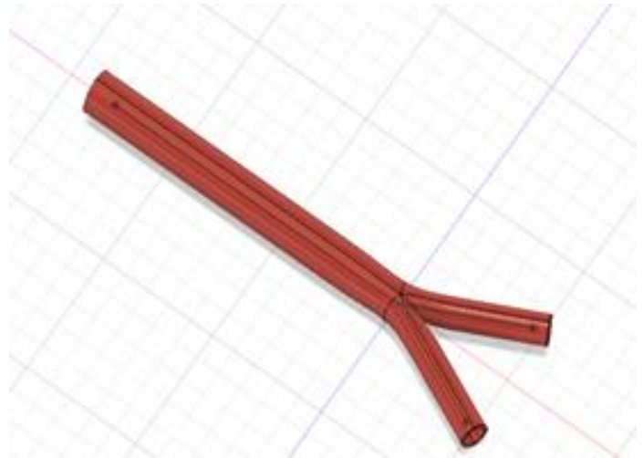
Supplementary Fig. 4. CAD model of the aorta and common iliac arteries. This image shows the CAD design for the phantom aorta.
