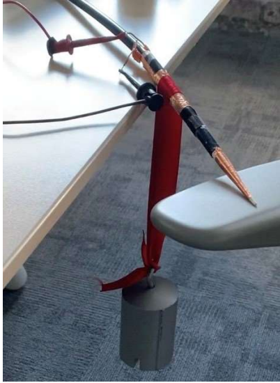
Fig. 3. Experimental set-up for measuring the voltage response to force for the FSR attached to a Cook Aortic Endograft. Known weights were hung on the sensor and the voltage output of the FSR was recorded.
