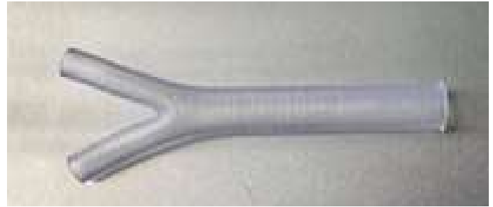
Fig. 2. 3D printed phantom of the AA and CIAs. The physiologically accurate dimensions for the phantom were determined from literature. Elastic 50A resin was used to print the phantom.
