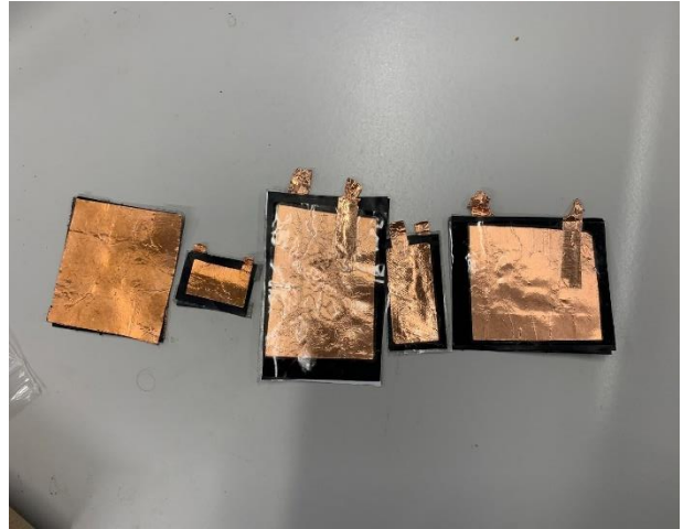
Supplementary Fig. 3. Force sensor iterations with a flat configuration. Multiple iterations of force sensing resistors in a flat configuration.
