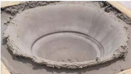
Fig 8.2.1 – Image depicting clay BFD from high speed testing
