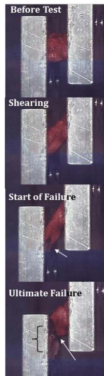
Fig 7.2.1 - This figure shows a time lapse of a sample failing in shear. The top picture shows the sample before the start of the test. The bottom picture shows the sample at the end of the test. The white arrows indicate the area where failure occurs.
