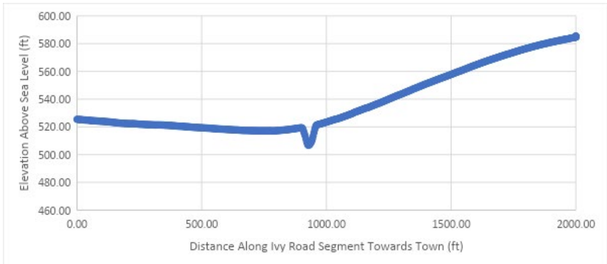
Figure 13: Graph showing distance along roadway versus the elevation above sea level. This is for the entire segment shown above.
