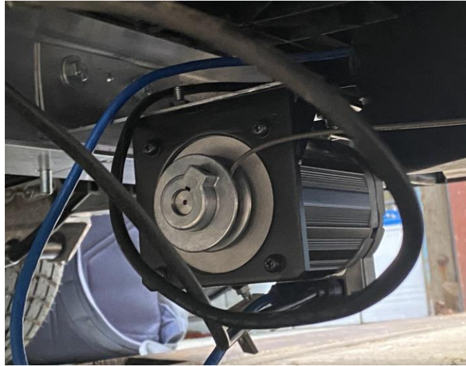
Figure 17: ClearPath Servo motor used for braking system on golf cart 789 with motor mount attaching it to the steel bracket underneath the cart.
