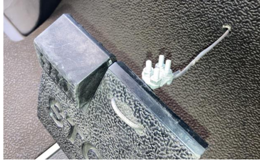
Figure 2: Attachment of the airline cable to the brake pedal of Cart 788 that allows for the pedal to be pulled when the brake motor is engaged.
