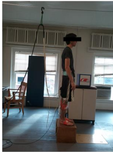
Figure C6. Overhead wiring system allowing free movement of the participant during the activity.
