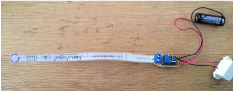
Figure 3.1b. Auditory biofeedback device inserted in a shoe at the head of the 5 th metatarsal
