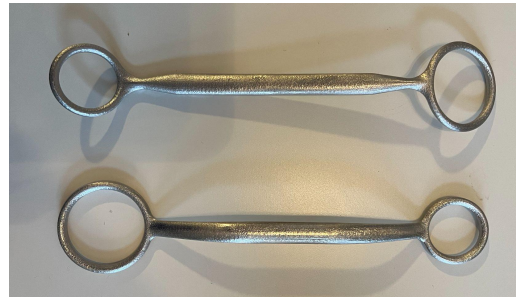
Figure 3. Polished DMLS Printed Prototypes. Stainless-steel devices after supports are removed and devices are polished.
