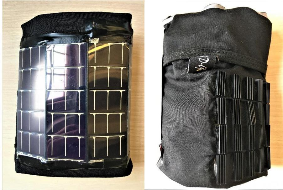
**Figure 6.8 Physical integration with an armband.**
