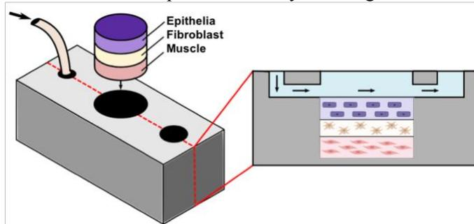
**Fig. 1. Overall device schematic.** An overview of the design concept and cross-sectional view of its components: a cell culture chamber to incorporate vertically-stacked hydrogels with three vaginal cell types, a port for tubing attachment to supply media through a microfluidic channel across the surface of such chamber, and a reservoir to collect the excess fluid after delivery.
