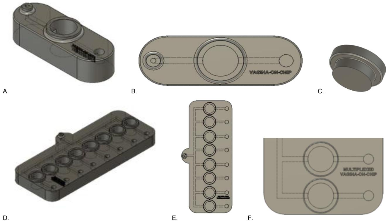
**Fig. 7. Final design & multiplexed platform.** (7A) Final CAD model of the vertical design including adjusted chamber dimension and a raised port for lid attachment. (7B) Top view of final CAD model, illustrates “VAGINA-ON-CHIP” inscription (7C) CAD model of removable lid (7D) Final CAD design of multiplexed platform including eight cell culture chambers supplied by a single port for tubing attachment (7E) Top view of final multiplexed CAD model (7F) “MULTIPLIED VAGINA-ON-CHIP” inscription
