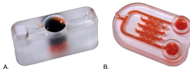
**Fig. 3. 3D printed prototypes.** (A) Printed vertical design with the successful layering of three agarose samples in the cell culture chamber. (B) Printed horizontal design with unintended leakage of agarose to all the channels. Both prototypes were loaded with multi-colored agarose to test hydrogel loading.
