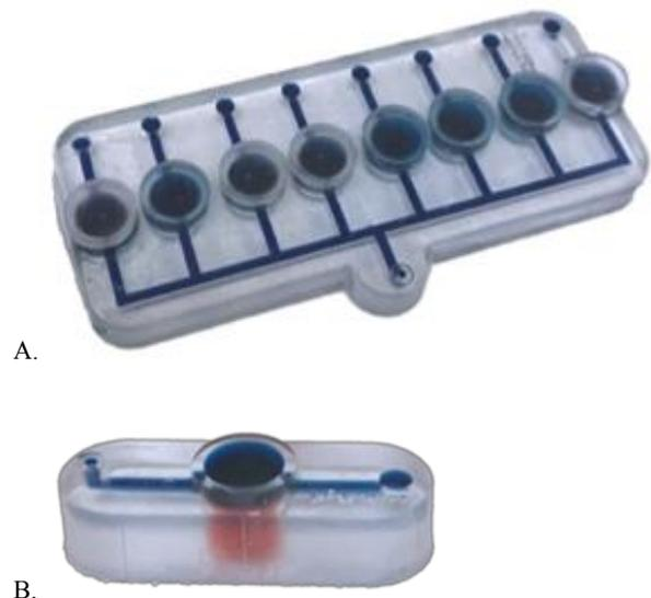
**Fig. 8. Final printed designs.** (8A) 3D-printed multiplexed device (8B) 3D-printed final single device with agarose to simulate hydrogel loading (red) and water (blue) to simulate cell media delivery through the channels and across the surface of the cell culture chamber.
