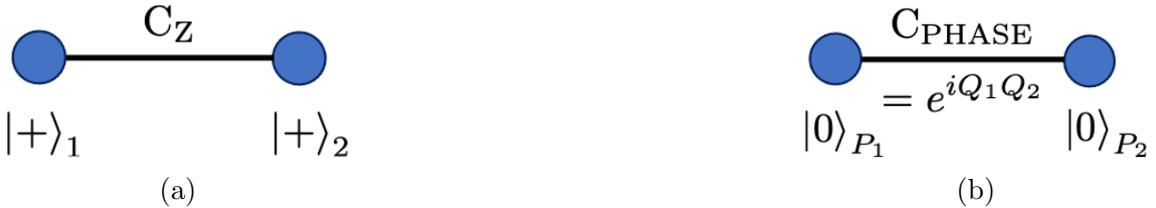
Figure 3.2: Graphical representation of a cluster state: (a) vertices denote qubits in the  $|+\rangle$  state, edges denote the  $C_Z$  gates; (b) vertices denote qumodes in the  $|0\rangle_P$  state, edges denote  $C_{\text{PHASE}}$  gates
