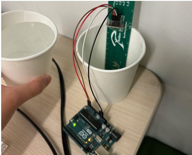
Figure 5: The setup for the LiDAR accuracy experiment. As shown, there is a ruler attached to the inside of the cup to verify ground-truth water height. The LiDAR sensor is attached above the water looking down towards the bottom of the cup.
