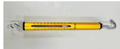
Fig. 5. Spring Balance Used in Force Testing
