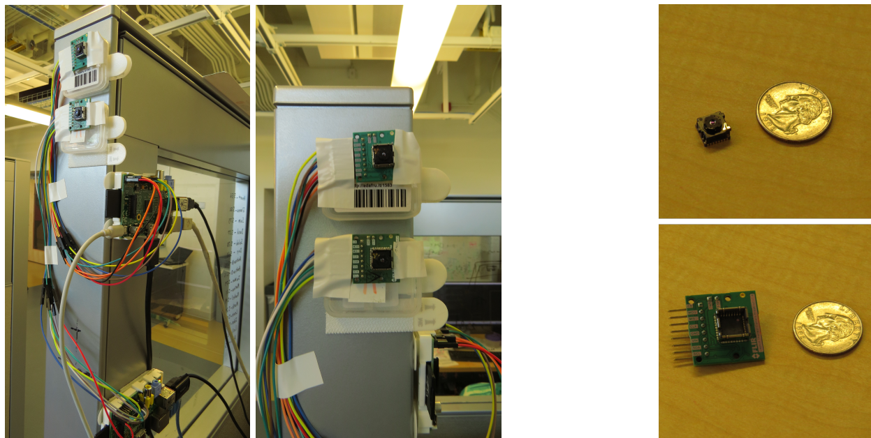
Figure 4.5: The two thermal cameras were placed vertically along a cubicle threshold and wired to two attached RaspberryPis (left). The FLIR imaging sensor and breakout board are shown to the right.
