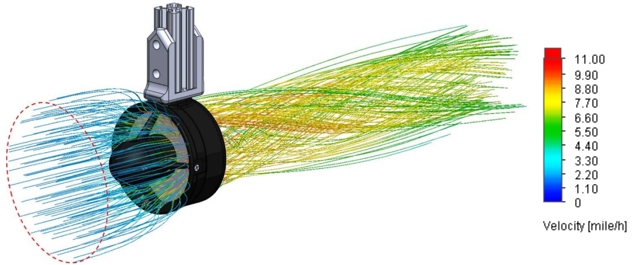
Figure 22: Thruster flow trajectories with velocity intensity (red circle is freestream diameter).
