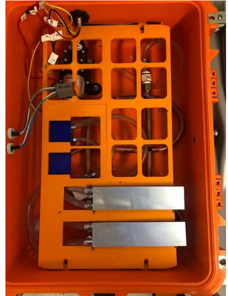
Cooling System and support structures
