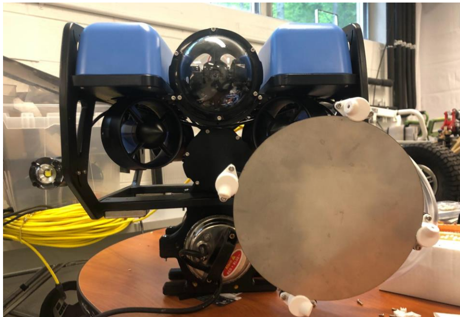
Figure 9: ROV Cleaning System.
