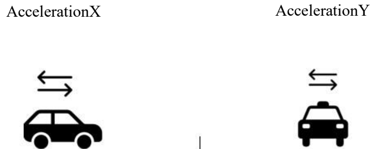
Figure 6. Illustration of AccelerationX (Forward/Backward) and AccelerationY (Lateral) movement in vehicle dynamics
