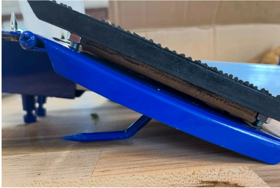
Fig. 39. Side view of final force sensor assembly
