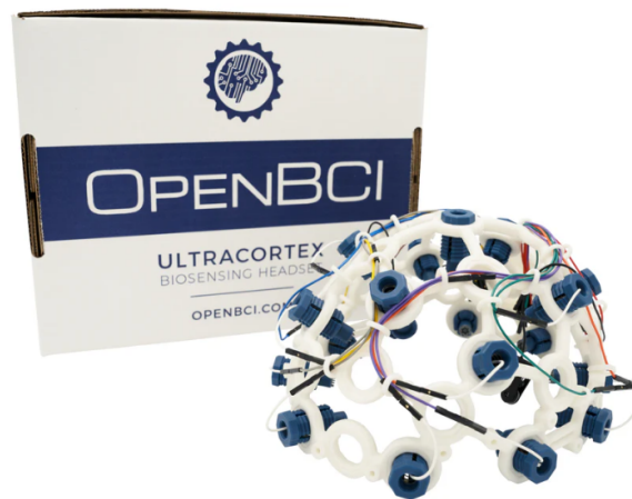
Fig. 4. OpenBCI EEG biosensing headset used for the project ( Ultracortex "Mark IV" EEG headset ).
