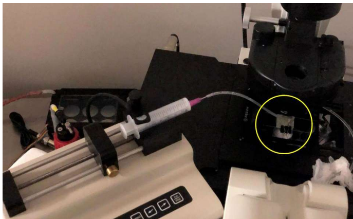
Fig. 2. Setup of 3D-printed prototype with syringe pump and microscope. The position of the 3D-printed device is indicated by the yellow circle.
