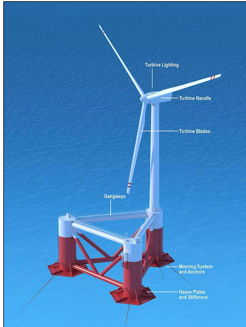
Figure 2. Principle Power Floating Offshore Wind Turbine Design (Image Source: Wikimedia Commons, 2020)
