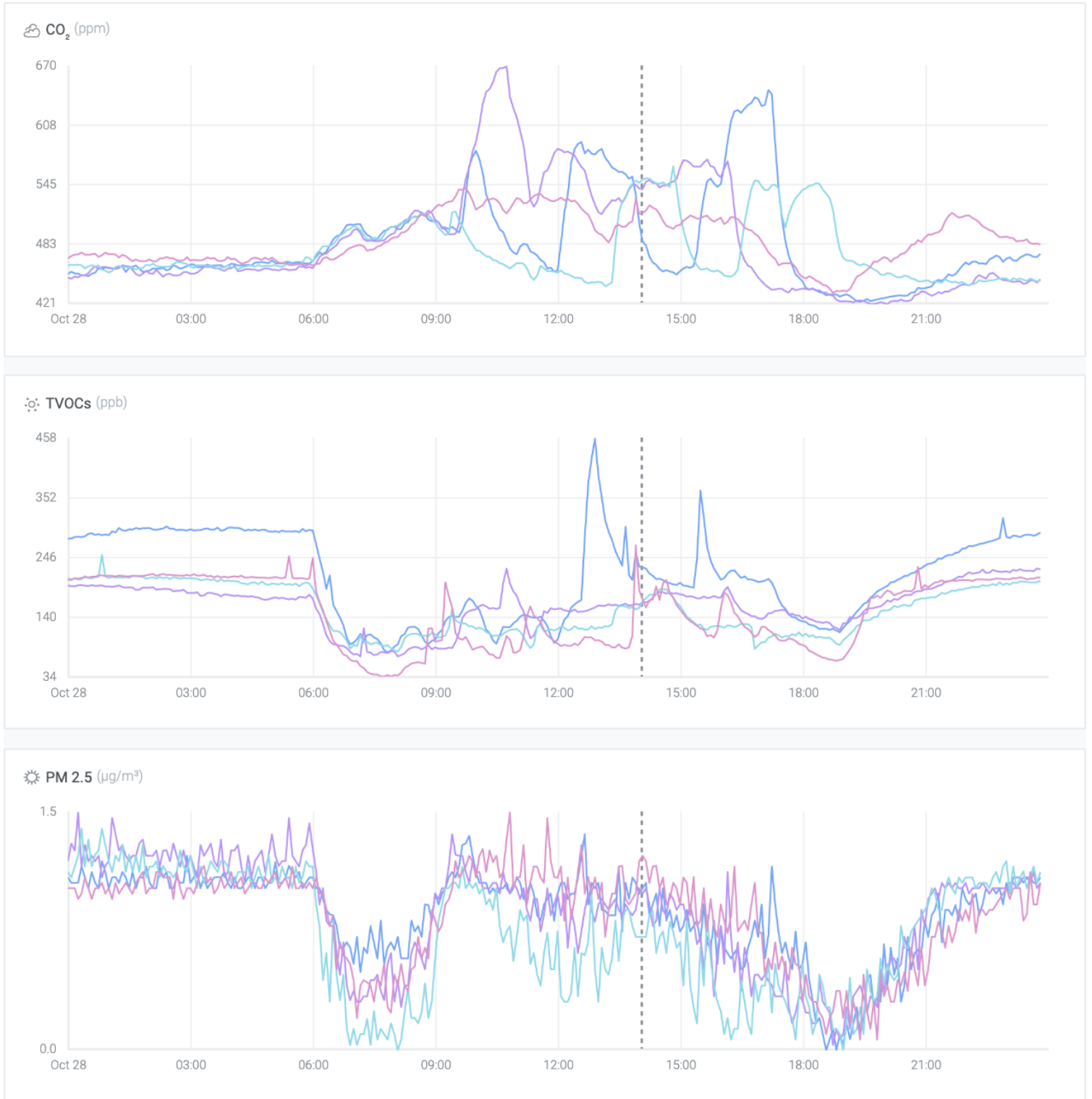
Figure 1. Measurements of Carbon Dioxide, TVOC, and PM 2.5 for four different rooms in Olsson Hall for October 28, 2021 (Awair, 2021)
