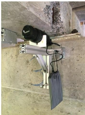
Figure 6.1. Camera mounted on bridge pier cap.
