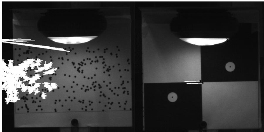
Figure 5.7. Lighting test: Sample optical flow tracking for speckle and checkerboard target patterns.
