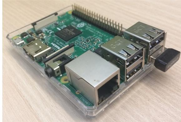
Figure 3.1. Raspberry Pi 3 Model B.
