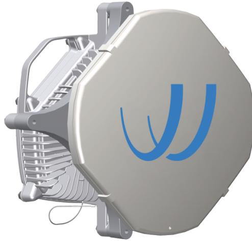
(b) An E-band (70/80GHz) millimeter wave system that claims 9.7Gbps capacity.
