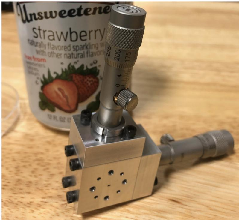
Figure 2.4: Assembled E-H Tuner
