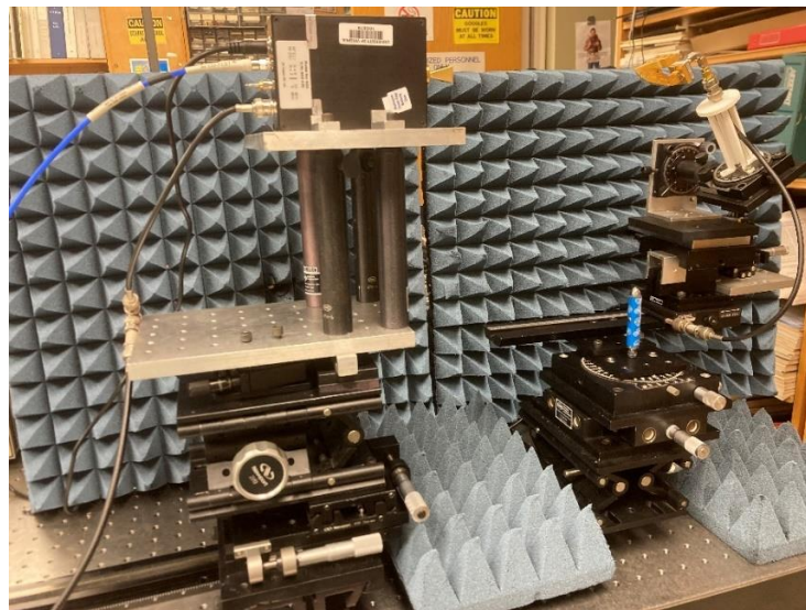
Figure 4.24 Picture of E-plane radiation pattern measurement setup of the WR5 quasi-Yagi.
