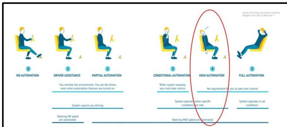
Fig. 1. Levels of Autonomy as Defined by The Society of Automotive Engineers (Wevolver, 2020)
