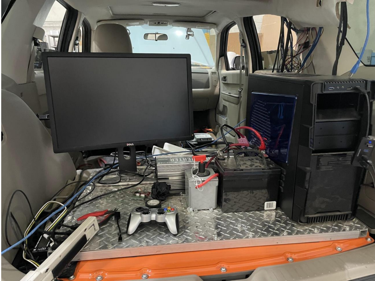
Fig. 28. From left to right, front to back: Power strip, computer monitor, joystick, power inverter, battery-kill switch, 12V battery, computer.
