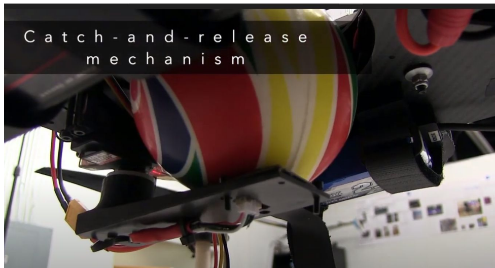
Figure 4: Drone catch-and-release mechanism
