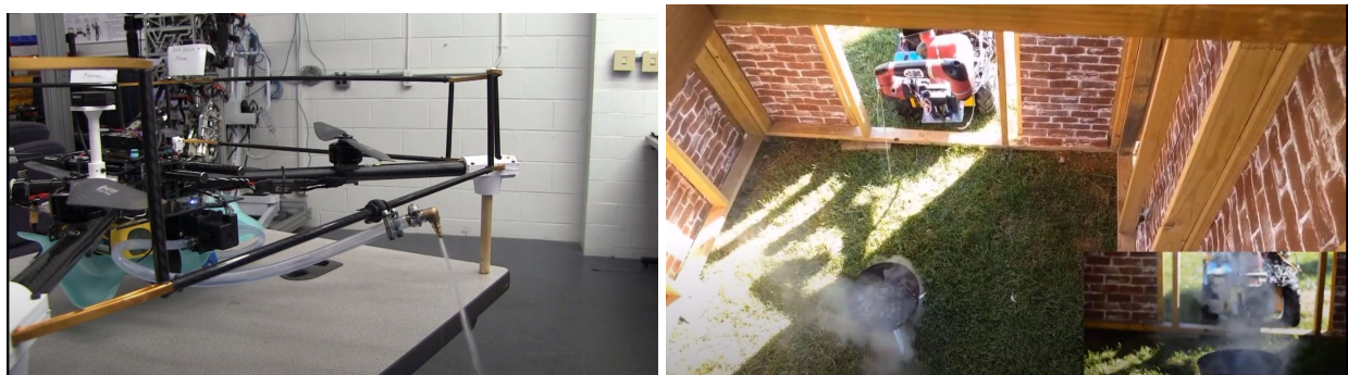
Figures 6 A: UAV with hose attachment, B: UGV expelling water at a simulated fire
