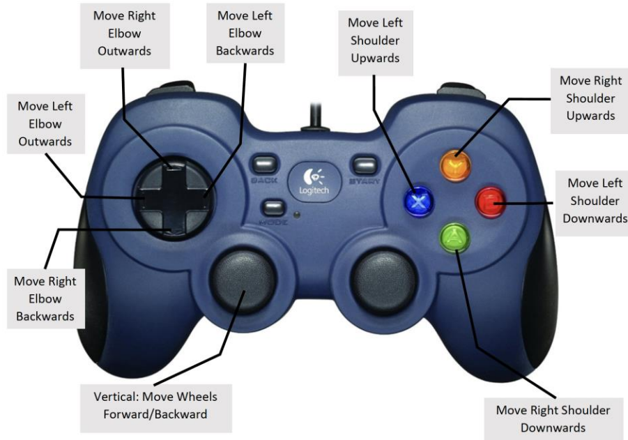
Figure 8: Controller Mapping Design
