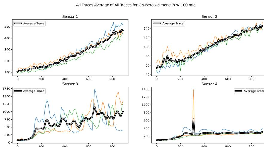
Figure 2.10: All Traces and Average Trace For Cis-Beta Ocimene  $100\mu L$  At Each Sensor
