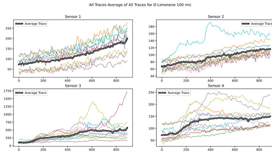
Figure 2.14: All Traces and Average Trace For D-Limonene 100 $\mu$ L At Each Sensor
