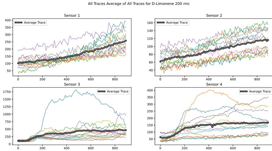
Figure 2.15: All Traces and Average Trace For D-Limonene  $200\mu L$  At Each Sensor
