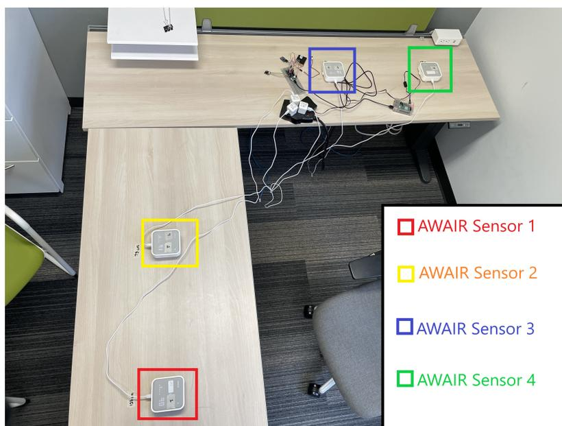
Figure 2.6: Image of room and setup
