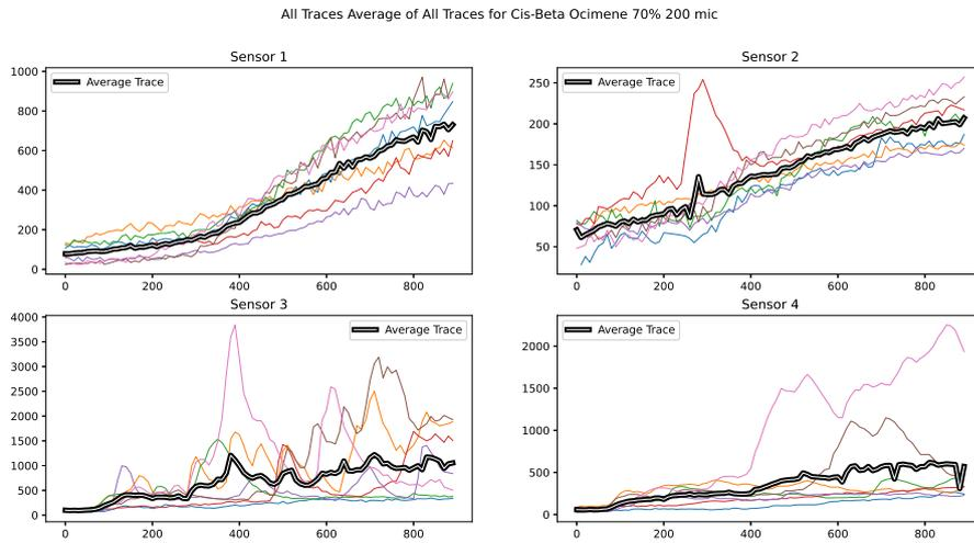
Figure 2.11: All Traces and Average Trace For Cis-Beta Ocimene  $200\mu L$  At Each Sensor
