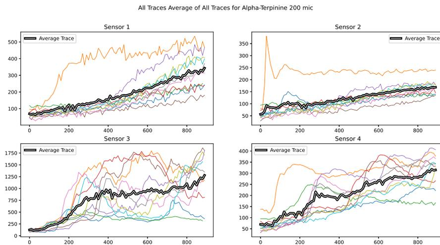
Figure 2.9: All Traces and Average Trace For Alpha-Terpinene  $200\mu L$  At Each Sensor
