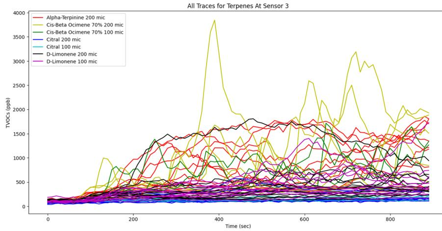
Figure 2.19: All Terpene Traces for Plant Terpenes At Sensor 3
