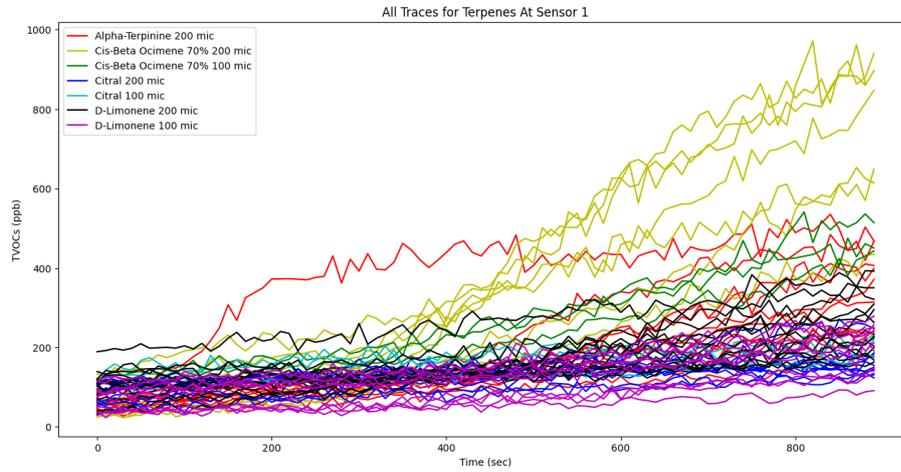
Figure 2.17: All Terpene Traces for Plant Terpenes At Sensor 1
