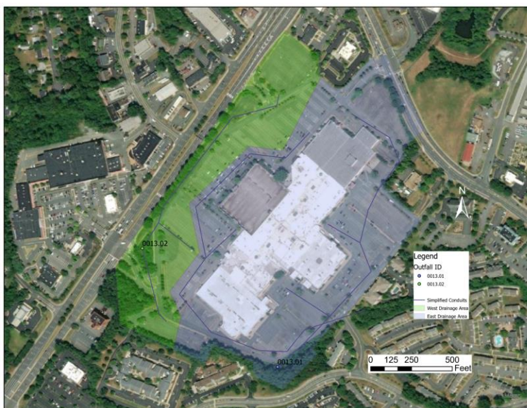
Figure 21. Drainage Areas to Site Outfalls.
