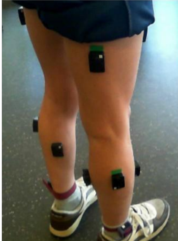
Figure 1: Trigno Avanti Sensors on a Participants Lower Limbs. Source: Boukhechba (2020)
