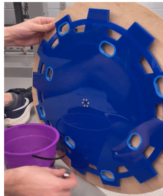
Fig. 11. Final test of gear functionality with pinballs
