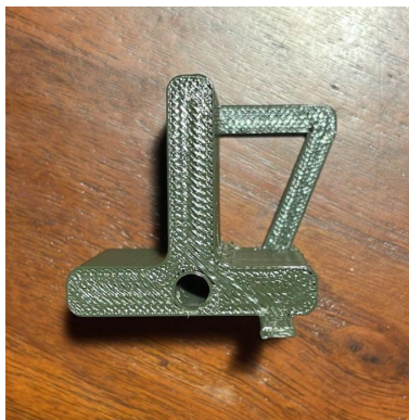
Fig. 23. Flipper with new preventative arm and tab (bottom)
