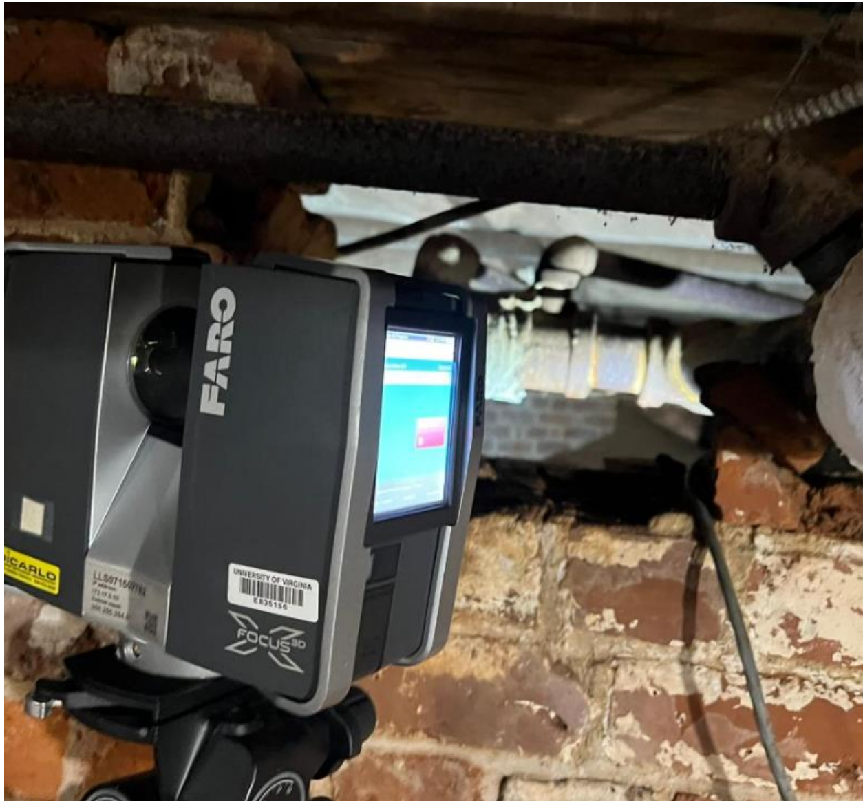
Figure 210: One of the holes viewing the inaccessible cellar from the accessible cellar. We set up a FARO Focus 3D LiDAR scanner in front of this hole to collect 3D data. Courtesy of Will Rourk.
