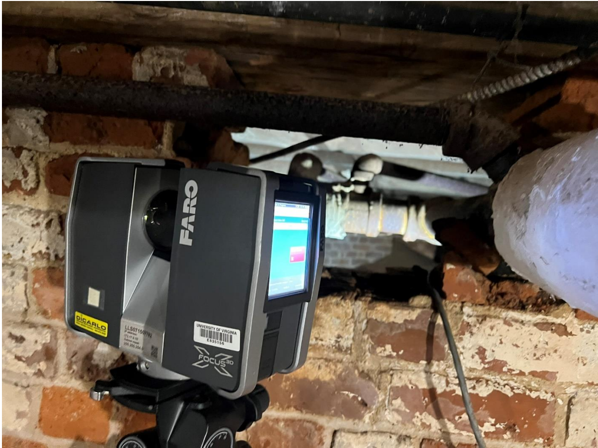
Figure 101: Photo taken of the hole in the cellar wall dividing Campaign One from Campaign Two, looking into the cellar under Campaign One. The diagonal wall with One-to-three bond is visible in the background, and the FARO Focus scanner is in the foreground. Photo taken by Will Rourk on March 3, 2025.
