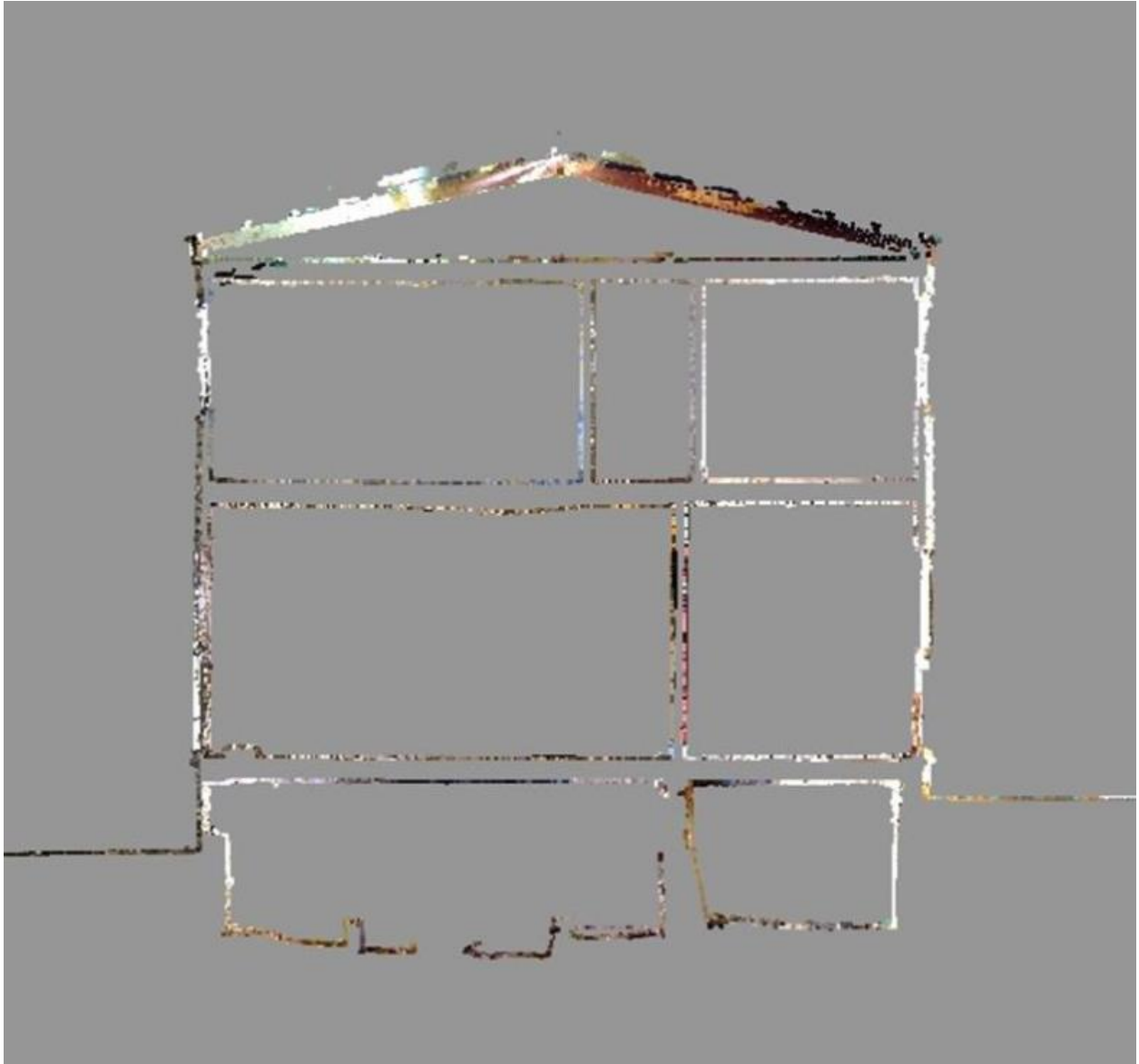
Figure 201: The section was taken from Campaign Two where the first floor was later modified and does not retain its original proportional relationships.
