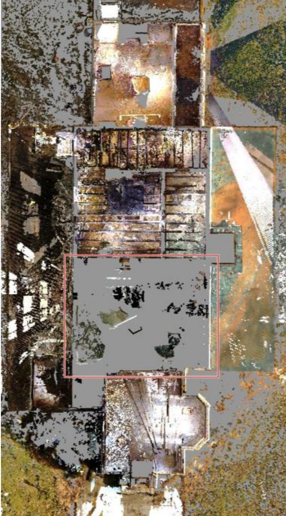
Figure 217: This floor plan view in Autodesk ReCap captures a view of all the data that we collected from in the inaccessible cellar.
