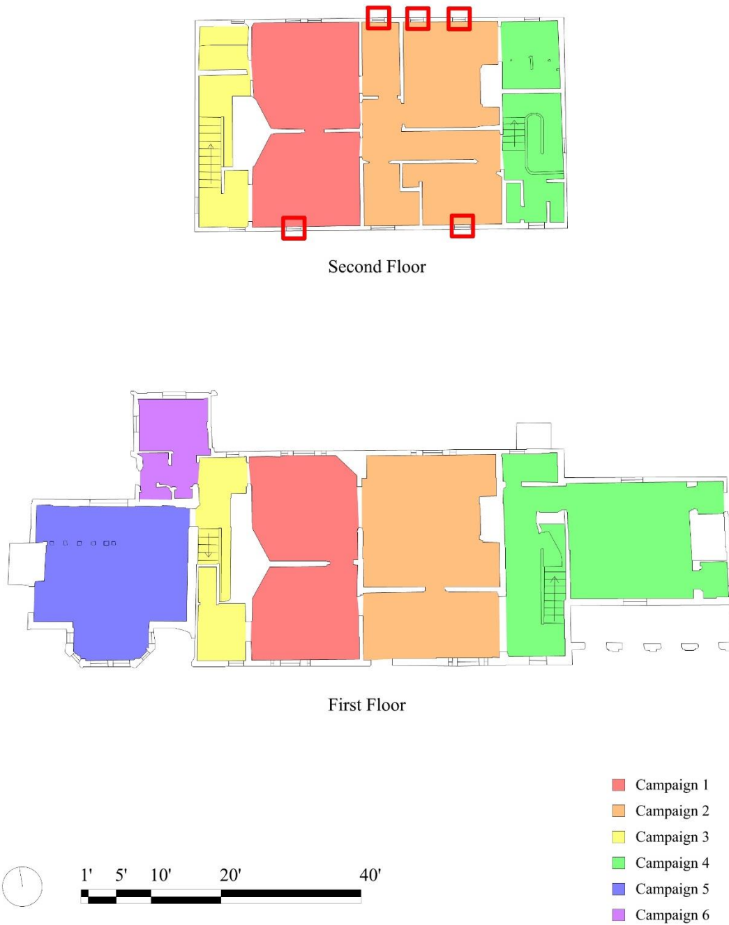
Figure 63: The location of the windows with matching trim that are in Campaign One and Campaign Two. The tripartite windows on the first floor are excluded since they are later additions. The double window on the north side of the second floor is also excluded. The southern window on the second floor of Campaign One matches the windows found on the second floor of Campaign Two, implying that those windows were added at the same time.
