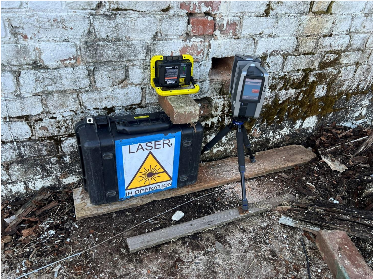
Figure 106: Photo of the hole in the northern foundation wall that views the inaccessible cellar. A 3D scan was taken from this location to capture the dimensions of the brick column seen in Figures 104 and 105. Photographed by Will Rourk on March 28, 2025.
