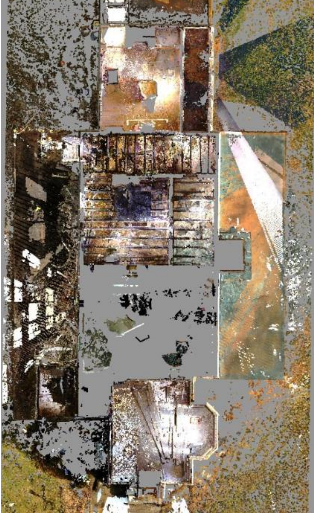
Figure 149: Another perspective of the floor plans of the two cellars. From this perspective, 3D data captured the joist information in the accessible cellar.
