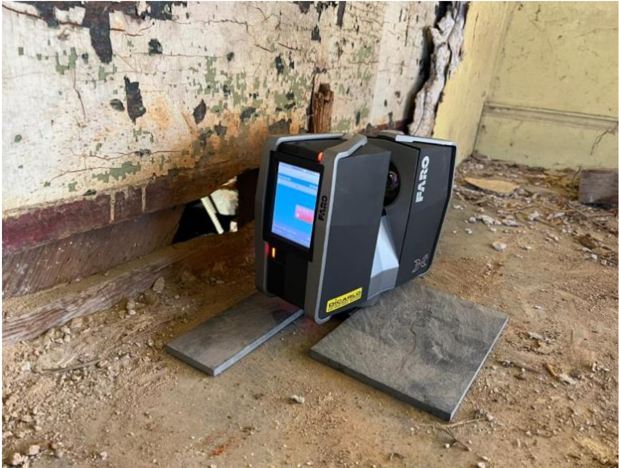
Figure 212: A photo of our scanner setup looking through the hole in the first-floor wing in Campaign Five viewing the inaccessible cellar. This scan was especially tricky because of how low the hole was. We stabilized the base of the scanner with tiles to ensure that the scanner did not move. This was experimental, but it worked well. Courtesy of Will Rourk.
