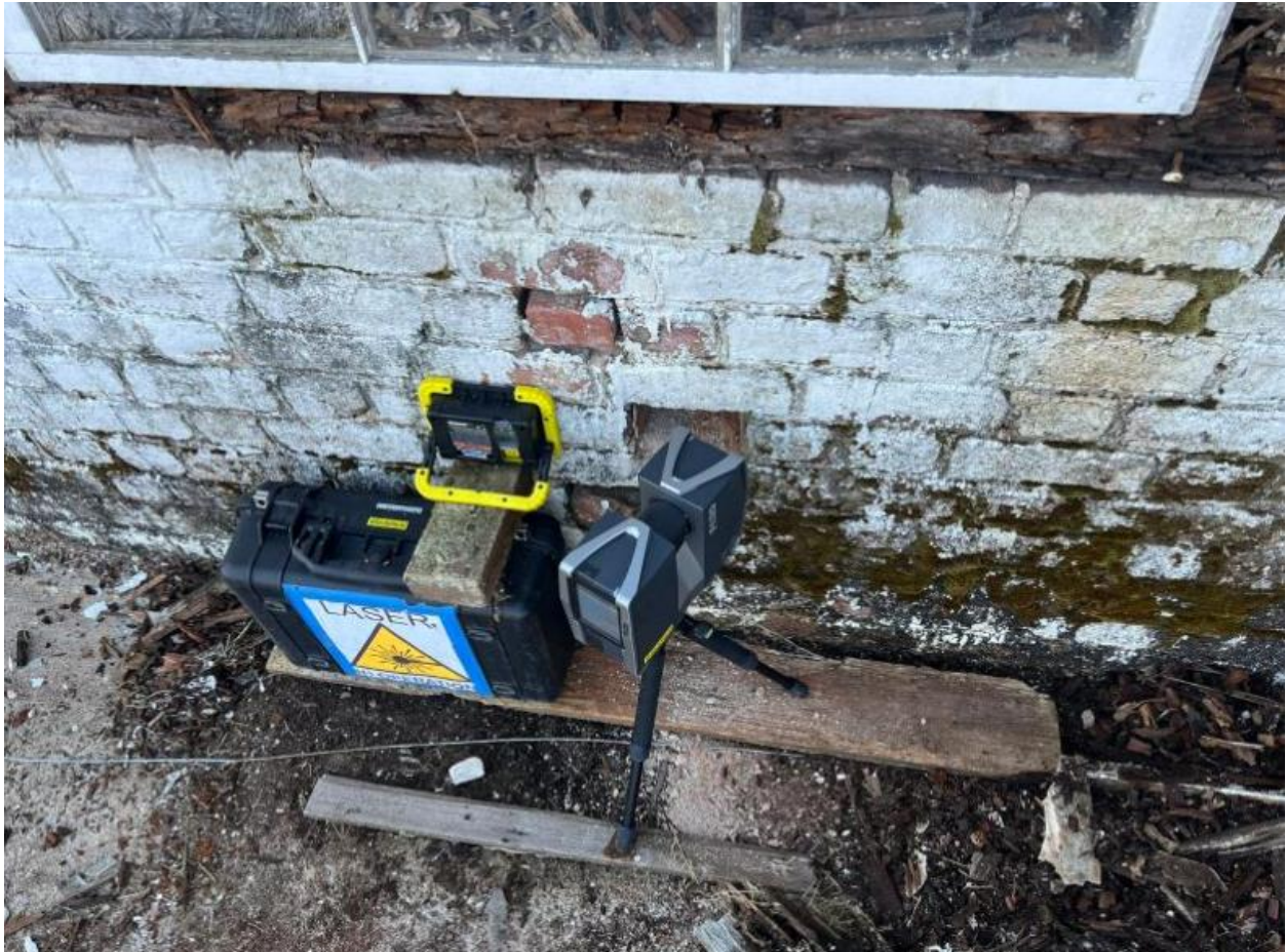
Figure 214: Photo of our scanner setup looking through the hole in the exterior brick wall into the inaccessible cellar. This hole was the smallest hole that we used, so it was challenging to position the scanner perfectly to gather as much data as possible. Courtesy of Will Rourk.
