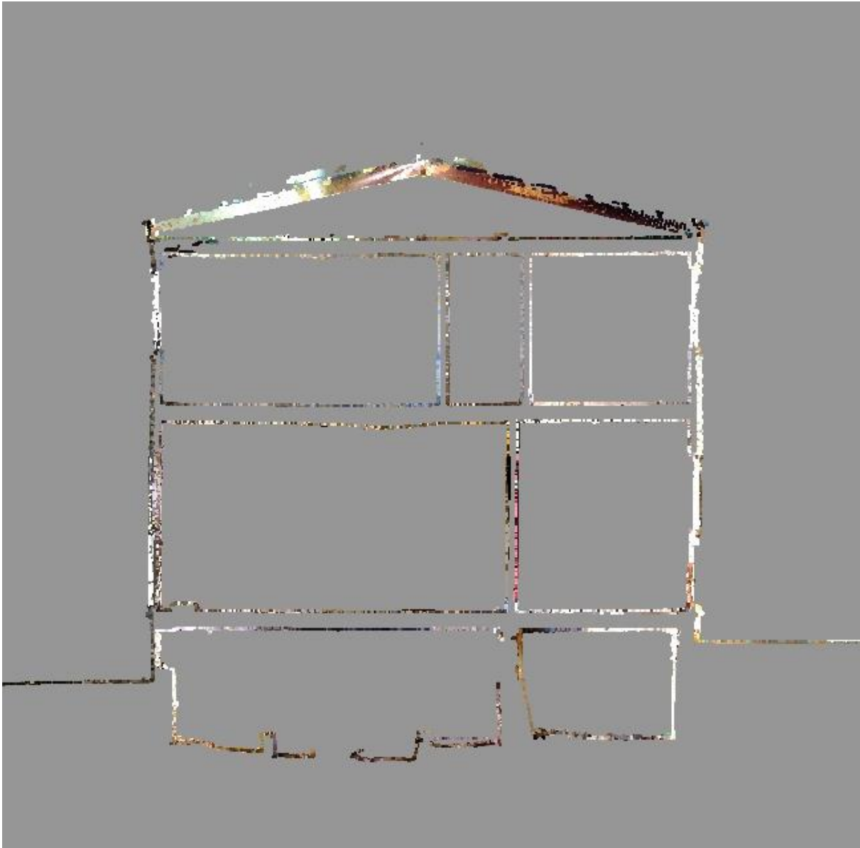
Figure 97: Section view of Campaign Two, facing East. In Campaign Two the layouts of the first and second floors do not share any relationship with each other, and the dividing walls on the second floor do not align with the wall on the first floor.
