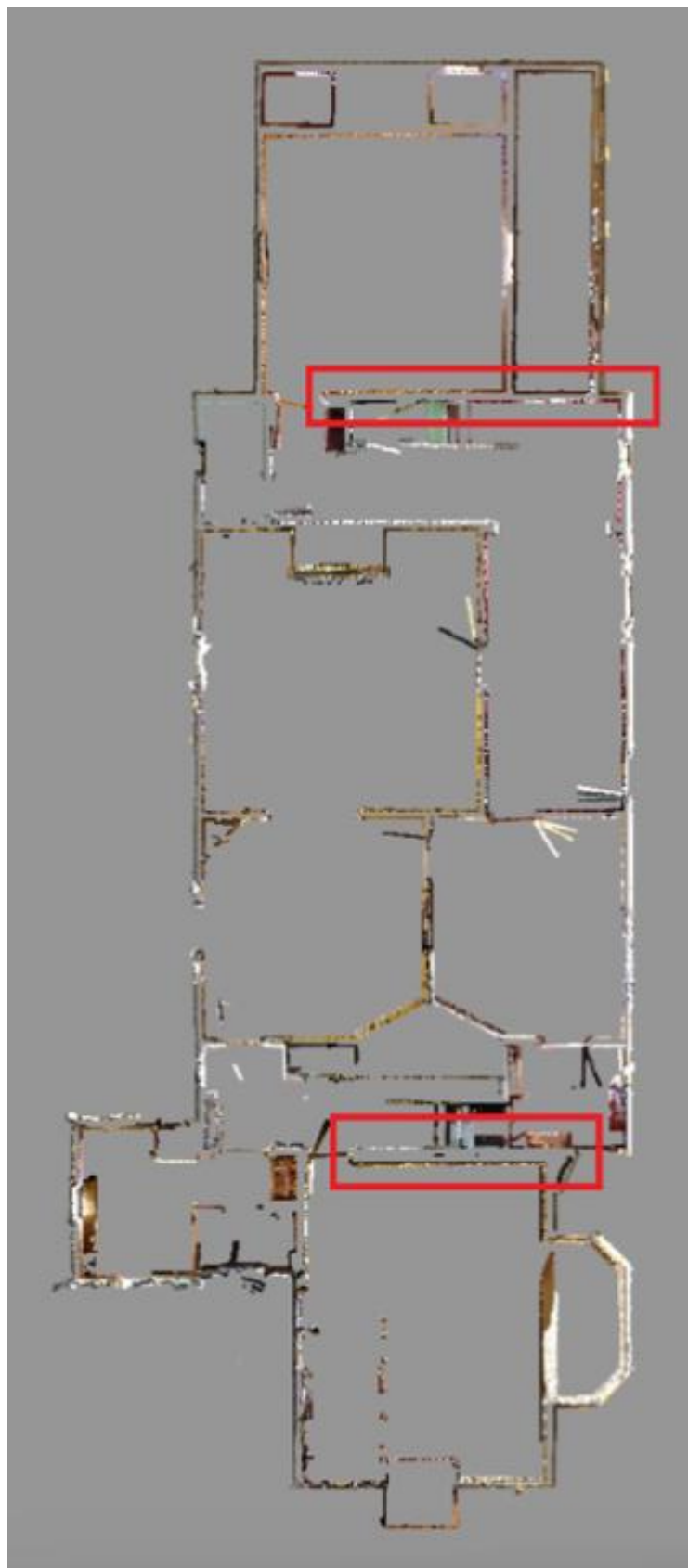
Figure 206: The location of the two walls joining the wings to the main portion of the house. The hole in the Campaign Five wall is in the wing to the left, and that wall is twice as thick as the wall joining the right wing to the house.
