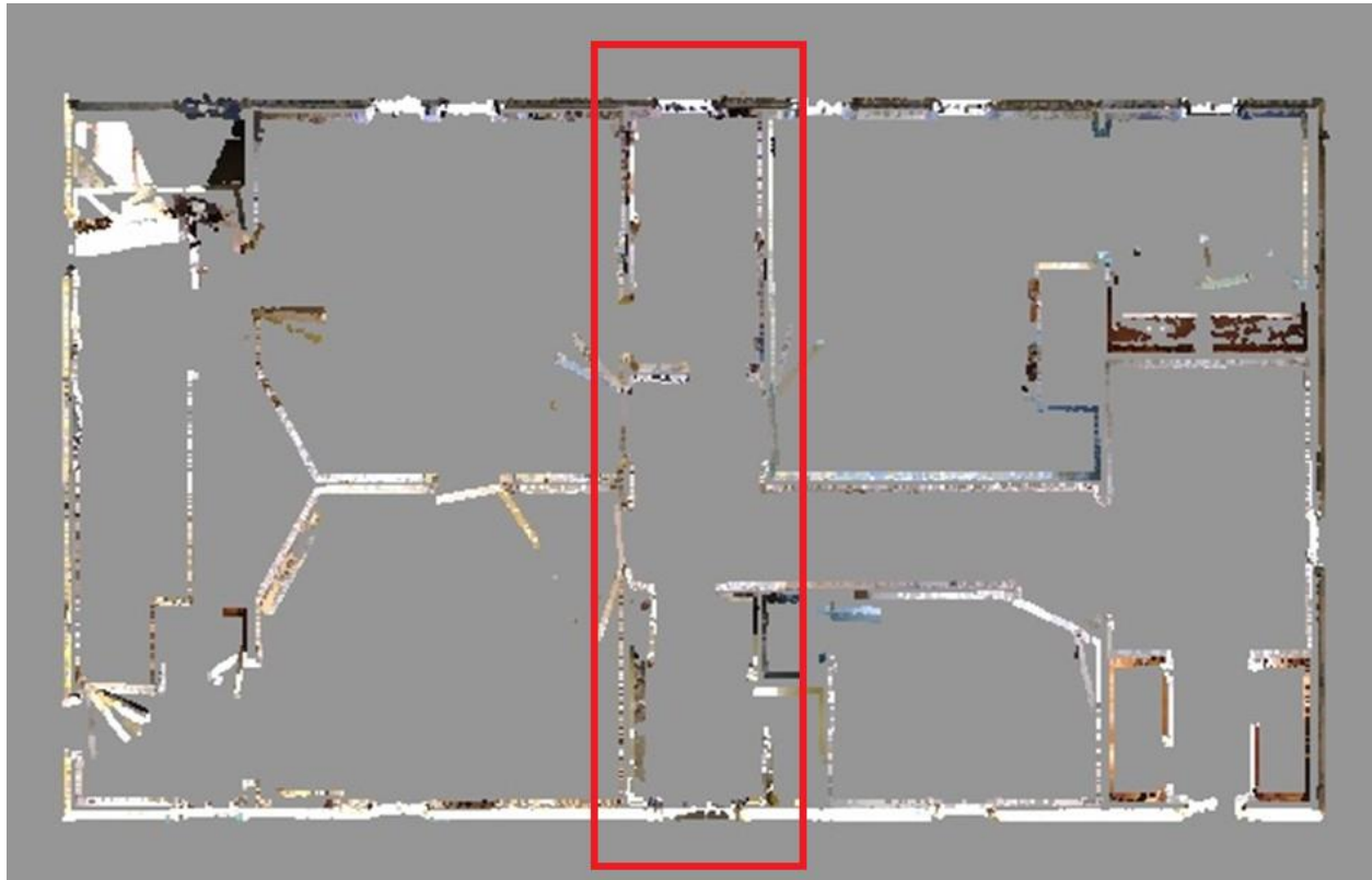
Figure 95: The location of a central passage on the second floor, which was later enclosed on both ends to create smaller rooms. Shown on the second-floor plan generated by 3D data.
