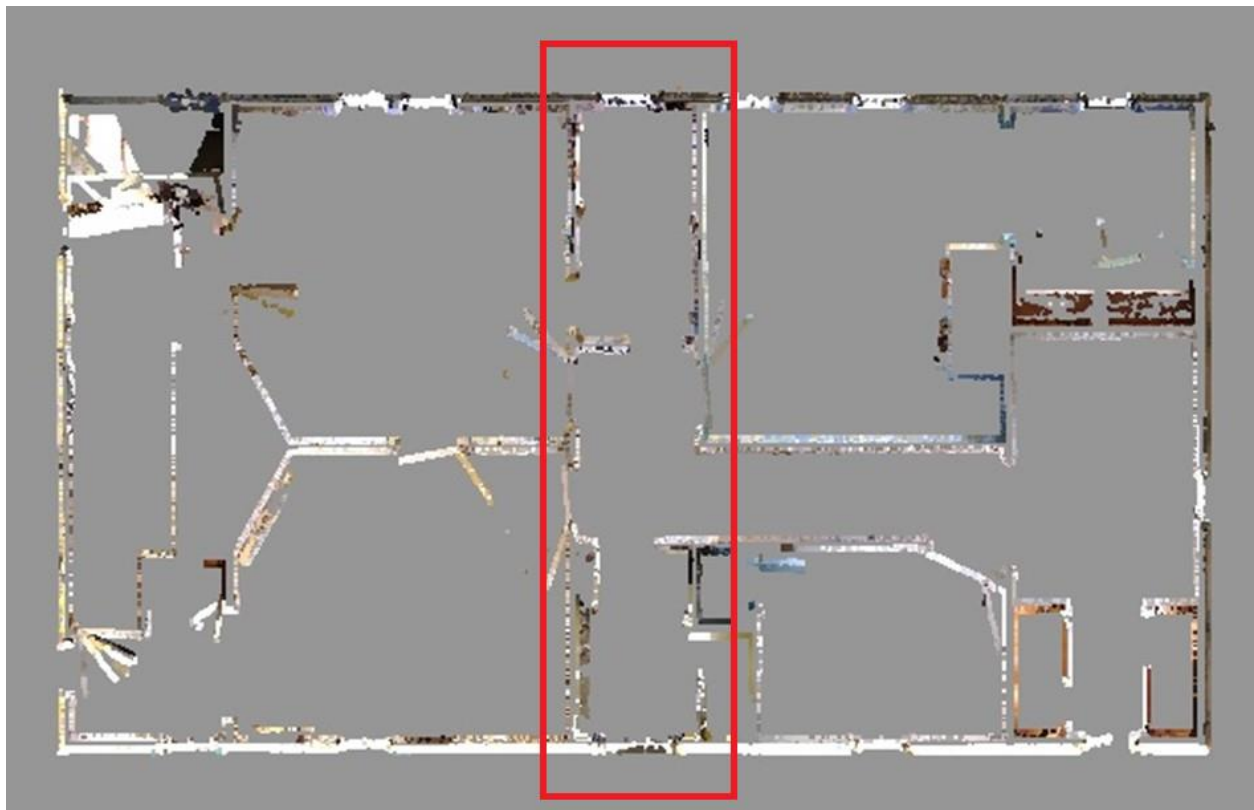
Figure 198: A view of the second-floor plan of Sylvania generated from 3D data with the location of the central passage highlighted in red.
