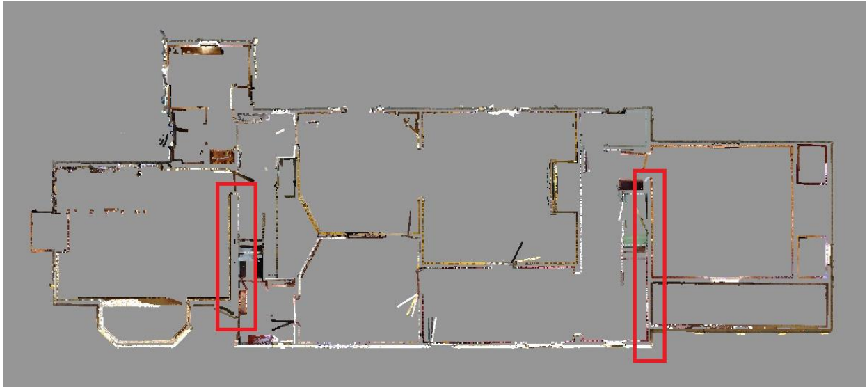
Figure 137: The thicknesses of walls joining the side wings to the main block of the house, shown on the first-floor plan generated by 3D data. The data reveals that the wall dividing Campaign Three and the west wing(left) is much thicker than the wall dividing Campaign Four's stair hall and the east wing(right).
