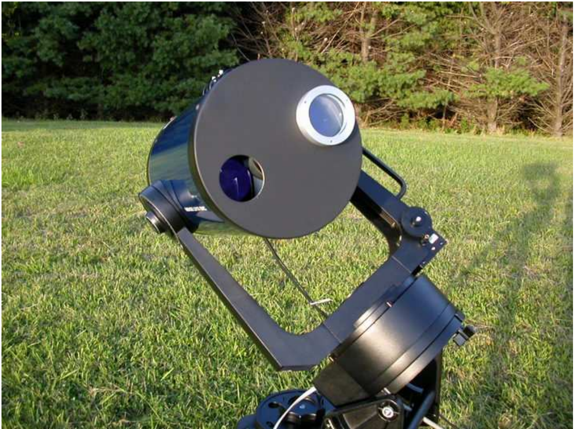
Fig. 1.5.— The Meade LX-200 DIMM Telescope equipped with an aperture mask. One aperture is installed with a 1' BK-7 wedge prism and the other is an empty opening.
