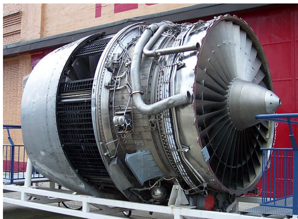
Fig. 9-1. Engine used on the Material Girl. Two Rolls-Royce RB211 engines on Material Girl. They are located 17 ft from the center line as shown by Figure 9-2.
