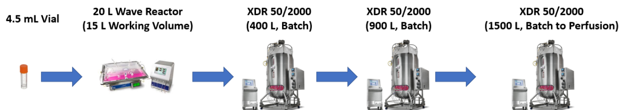
Figure 4.2. Scale-up equipment and working volume requirements from 4.5 mL vial to 1500 L perfusion reactor ( Xcellerex™ XDR Cell Culture Bioreactor Systems , 2020).
