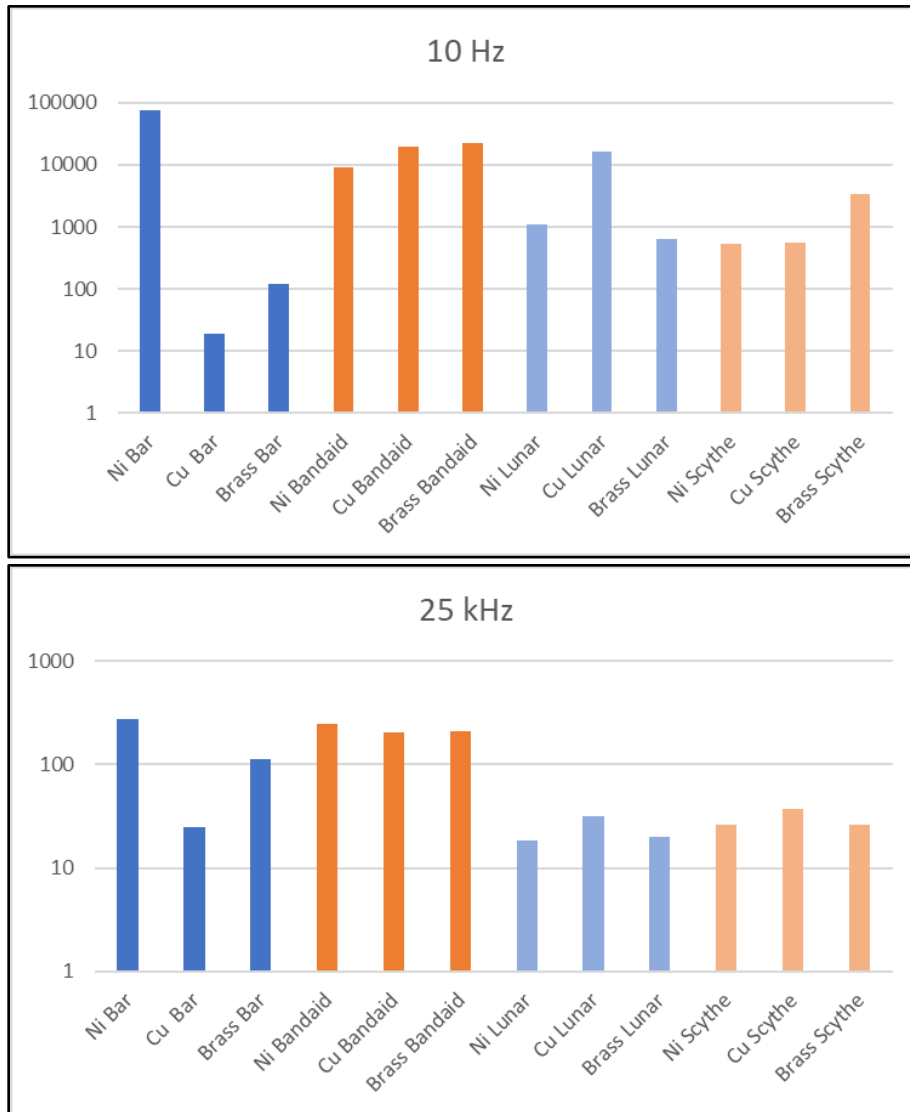
Figure 10. Impedance ratios sorted by geometries, separated frequencies 10 Hz (top) and 25kHz (bottom).
