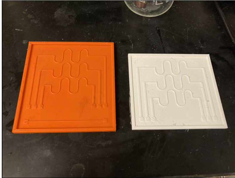
Figure 3. Two sensor molds, including the last iteration with a reference channel on the left.
