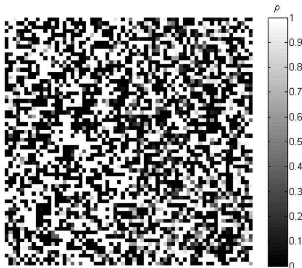
Figure 4.5: Example fingerprint for an SRAM array [117]. Across a chip, the skews of the SRAM cells produce a unique pattern where most cells are skewed toward 1 (black) or 0 (white), but some are close to 0.5, or are balanced (gray).
