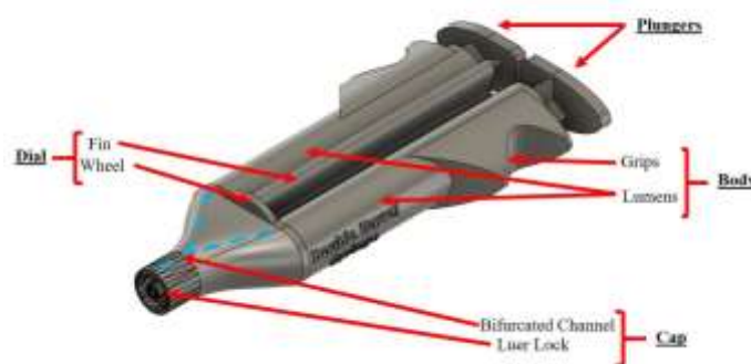
Figure 2: The five main components of our main design consist of the labelled “Cap”, “Dial”, “Body”, and “Plungers.” Additional features of the design include sub-components such as: “Fin”, “Wheel”, “Grips”, “Lumens”, “Bifurcated Channel”, and “Luer Lock.”
