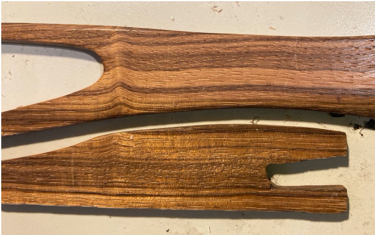
Figure 33: Comparing the two zebrawood tongues side by side, with grain matched to show position in the blank, 2025
