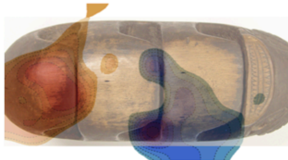
Figure 13: Radiation pattern of the second partial for a played tone of the highest plate of 1440 Hz, top view.
