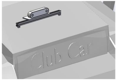
Figure 5: Draft of front-facing camera mount.
