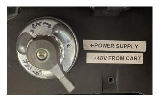
In the rear of the cart, on the left-hand panel, is an inverter. After the inverter is switched on, the computer and monitor may be turned on.
