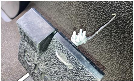
Figure 2. Airline cable secured to the brake pedal
