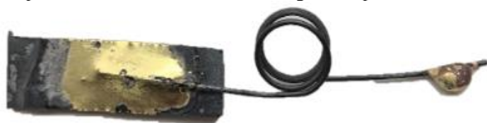
Figure 8: Brazed Coil Spring. The coil spring is brazed onto a small rectangular piece of steel as a test. Attempts to recreate the joint with specific pieces failed.
