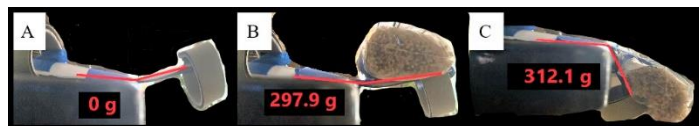
Figure 9A-C: Samples of images from thermoplastic device testing. These figures, along with many others, were put into ImageJ where the angle was calculated and recorded for later inclusion in a force graph. Figure A shows the initial position. Figure B shows the last measurement before device failure, while Figure C shows the first point of failure.
