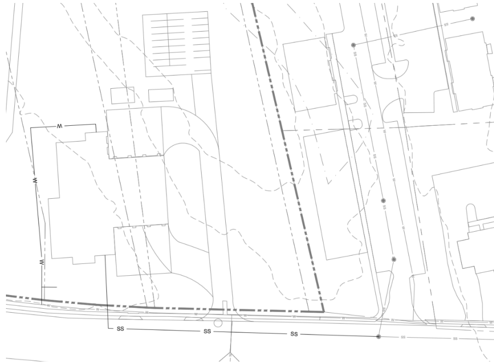
Figure 2.2.8.1: Plan view of utilities layout for water pipes (W) and sanitary sewers (SS), with connections on nearby parcels.
