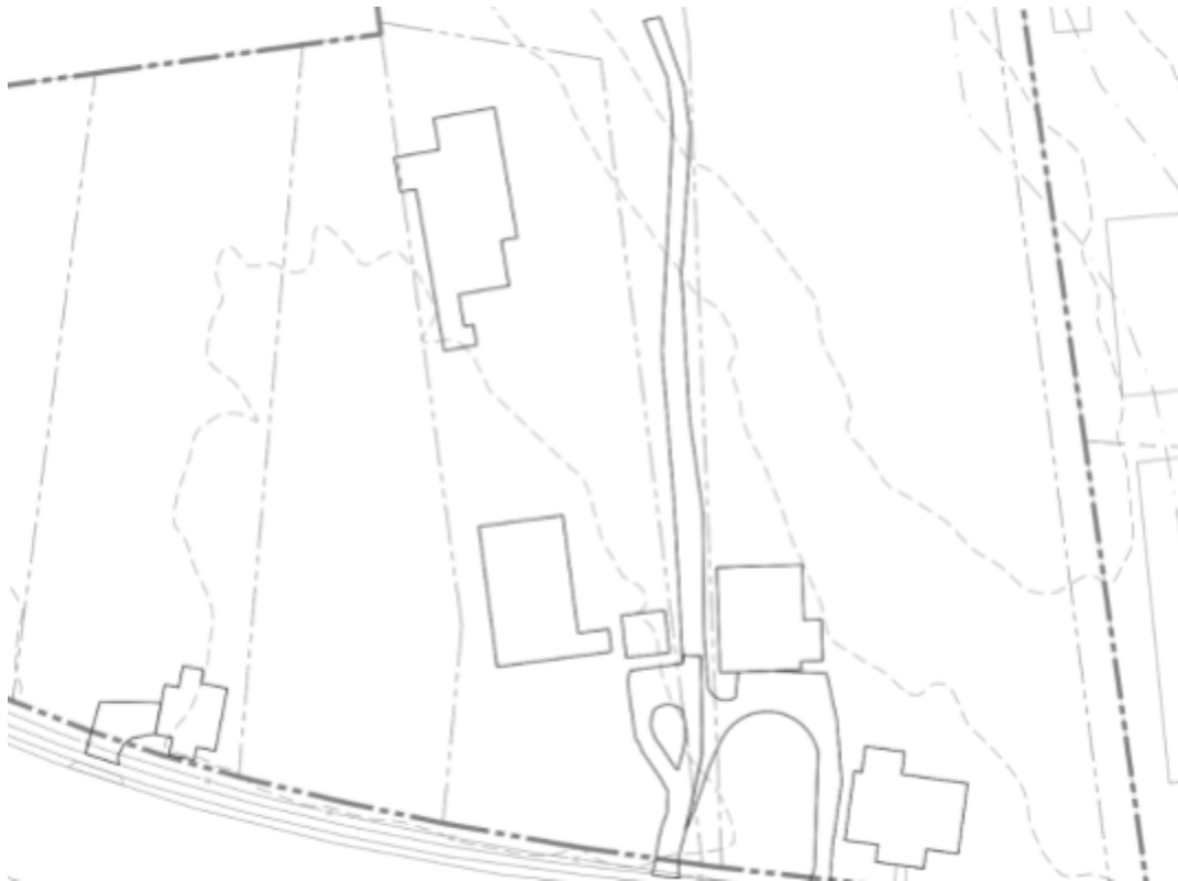
Figure 2.2.3.1: Demolition plan view, all buildings, roadways, and features outlined in bold will be demolished at the start of the construction phase.
