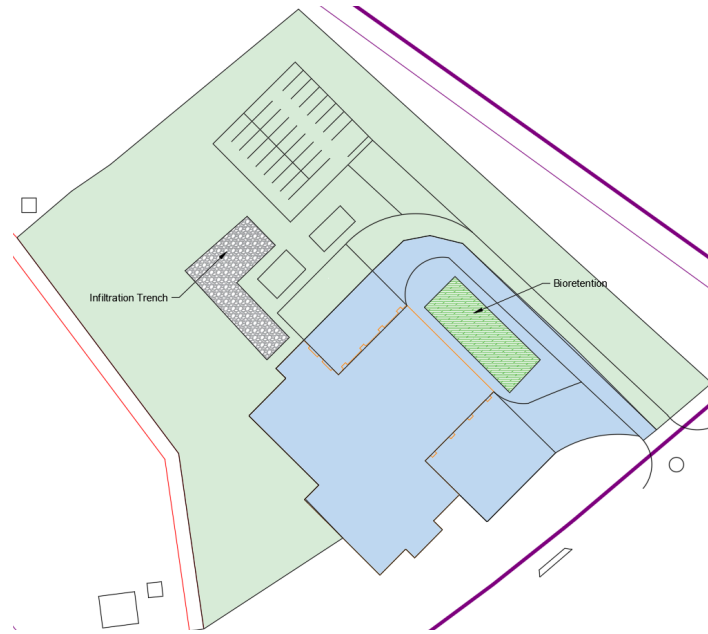
Figure 2.2.7.1: Plan view of BMPs for stormwater management. The bioretention has a surface area of 2300 ft 2 and the infiltration trench has a surface area of 2800 ft 2 . The green area (77,000 ft 2 or 1.8 acres) drains to the infiltration trench and the blue area (31,000 ft 2 or 0.7 acres) drains to the bioretention basin.
