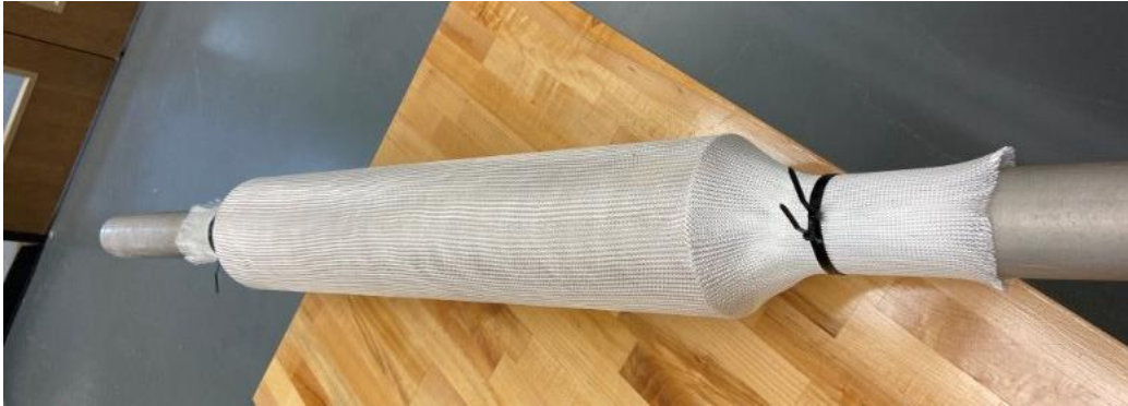
Figure 63. Fiberglass sleeve fixed over phenolic tubing.
