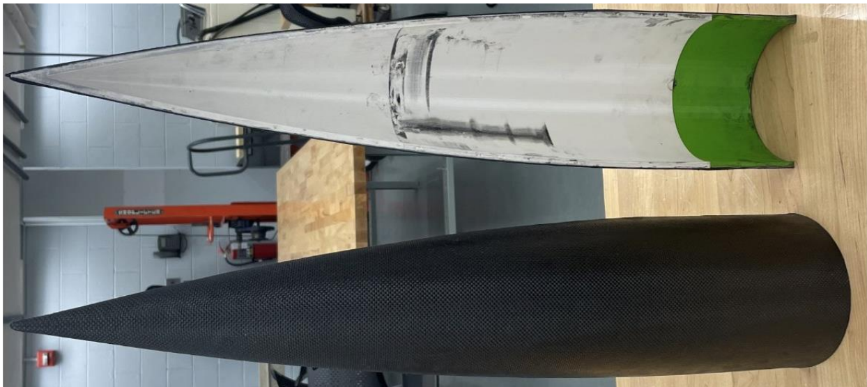
Figure 57. After 3 layers of CFRP wet layup
