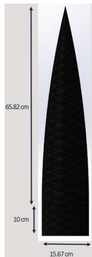
Figure 3. Final ogive nosecone design and dimensions.
