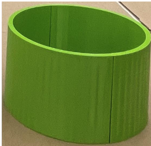
Figure 55. Extended nosecone mold (Height 10 cm)
